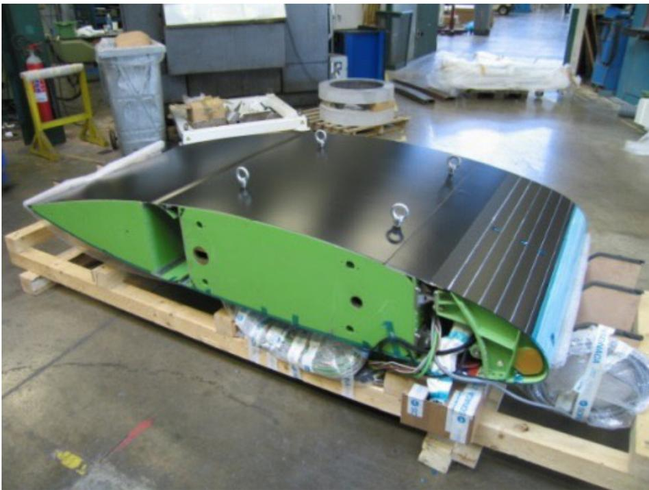
Fixed Leading Edge + Wing Box + Actuated Flap for military Wing section anti-icing test
